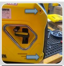
STEP 5: REMOVE THE SCREWS FROM THE LOCATIONS SHOWN
