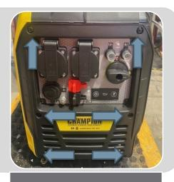
STEP 1: REMOVE THE SCREWS FROM THE LOCATIONS SHOWN STEP 2: REMOVE
