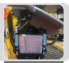
STEP 12: REMOVE 8MM BOLTS SHOWN TO FREE THE CONTROL UNIT
