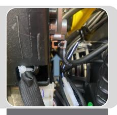
STEP 9: SLIDE THE CLIP DOWN THE FUEL PIPE AND REMOVE
