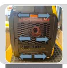
STEP 4: REMOVE THE SCREWS FROM THE LOCATIONS SHOWN, ONCE REMOVED PUT THIS PIECE TO ONE SIDE
