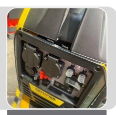
STEP 6: AFTER THE PREVIOUS STEP POP THE FRONT PANEL OUT OF THE CASING LIKE SHOWN ABOVE
